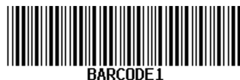
b) Code 39 symbol, representing the string *BARCODE1*
